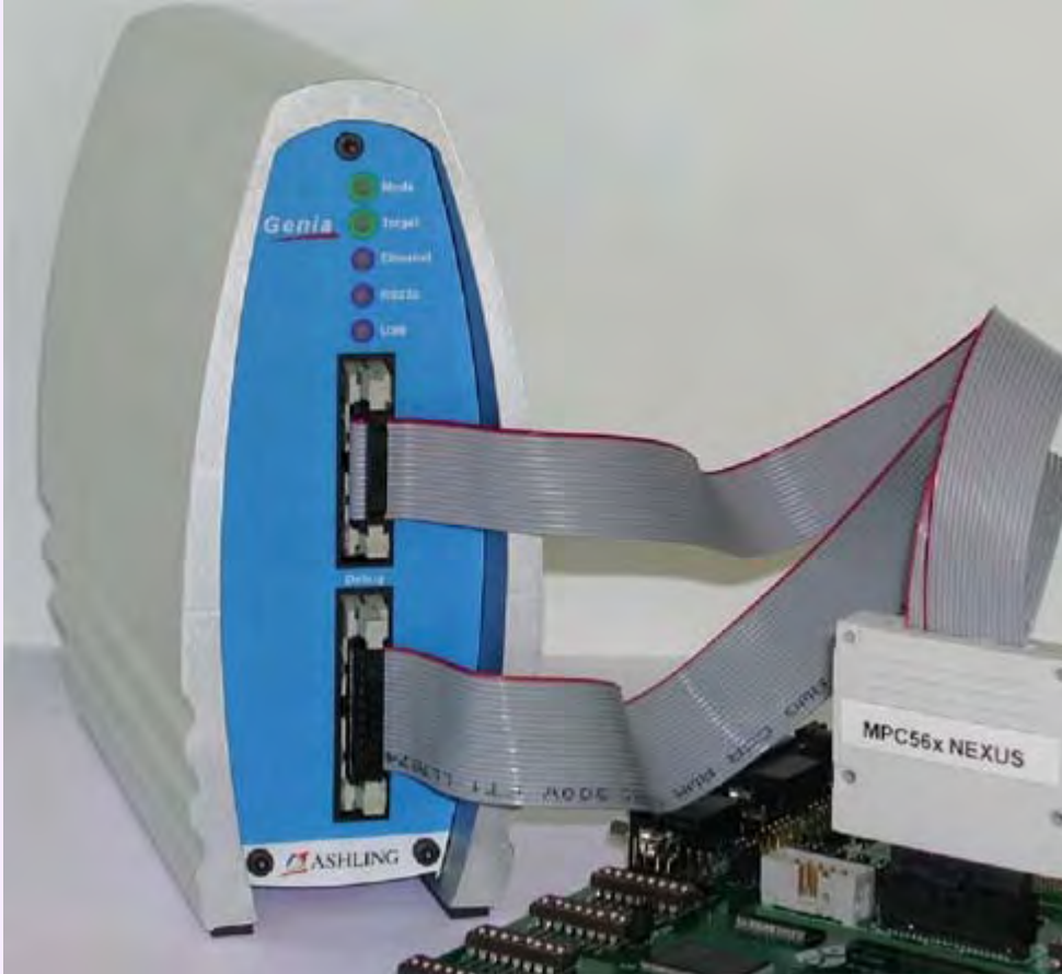
Ashling Genia NEXUS and BDM Emulator for MPC5554, MPC565 and MPC555 shown here connected to Freescale's MPC565 development board using the NEXUS (IEEE-ISTO-5001™) interface
